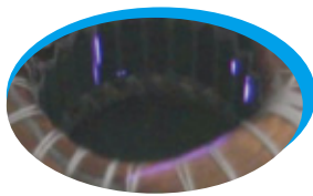
Corona discharge in motor
