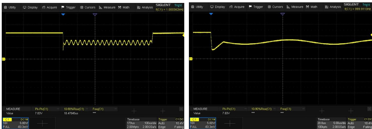
Figure 6: cranking voltage measured across the EUT supply line
