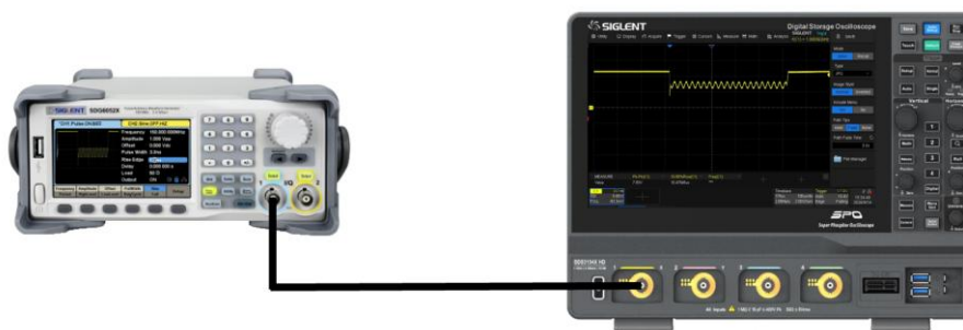
Figure 4: setup to adjust the output signal
