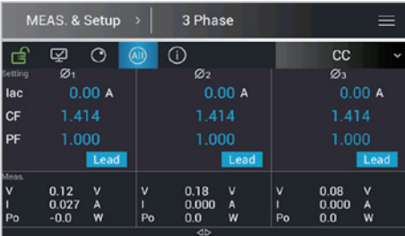
CC Mode Main Screen (Three Phase)
