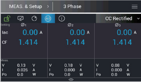
CC Rectified Mode (Three Phase)
