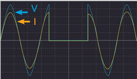
Voltage Interruption Load Testing (CR Mode)
