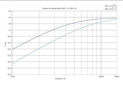
The high coupling factor of the EMCL-35 allows a test according to level 3 (10V) of IEC 61000-4-6 already at 10 kHz with the test generator CDG 7000-75-10.
