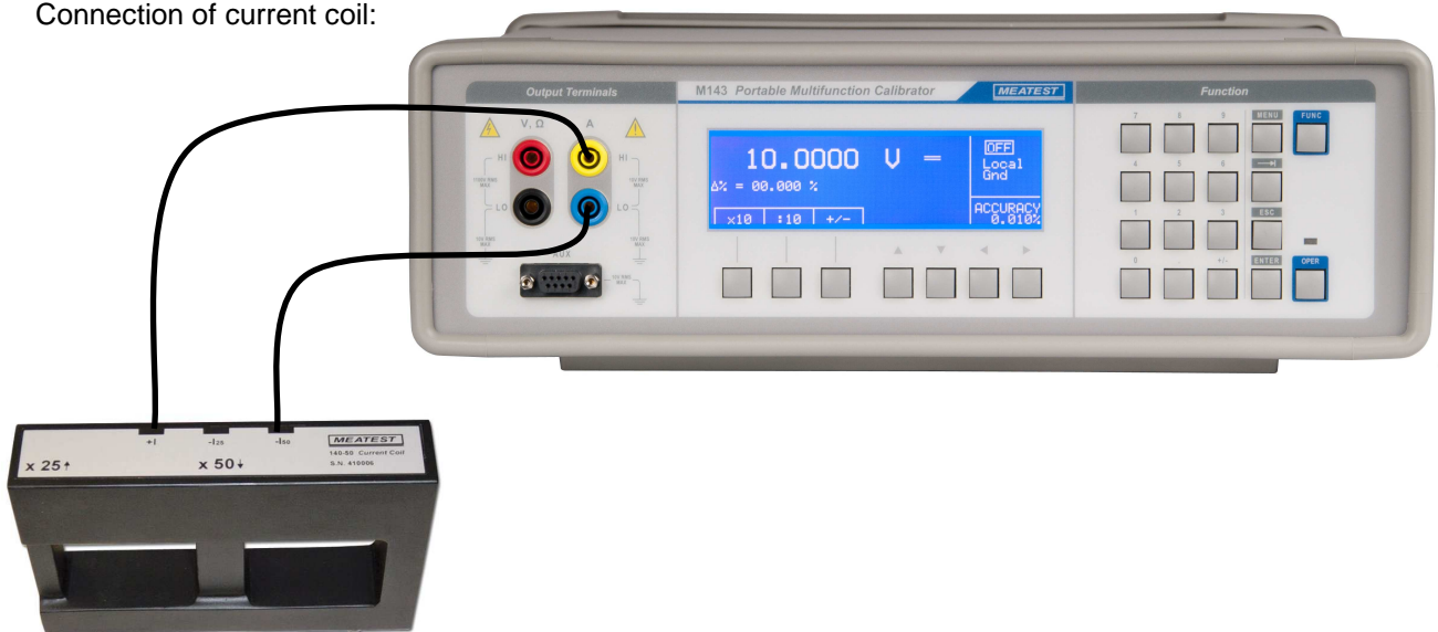
Fig. 25 Current coil connection
