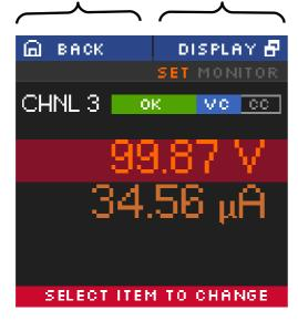
selected screen: set or measurements selected channel with its running and regulation state (constant voltage / constant current
