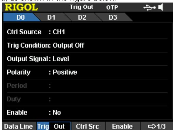
Figure 2-7 Trigger Output Setting Interface
