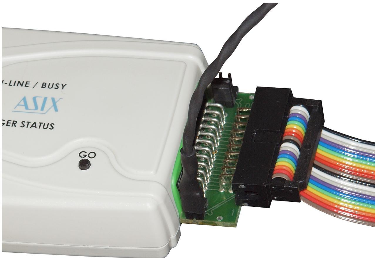
*Fig. 12: Using of the OSH-2 synchronization header*
